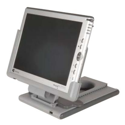
The Motion FlexDock, a desktop docking station, includes most of the tablet's peripheral device connectors.
