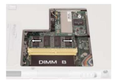
**10** If you are removing a memory module, pull the module out of the slot.
