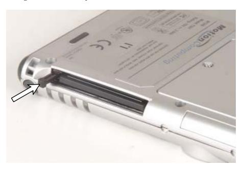
**2** Push the PC Card firmly into the PC Card slot label-side facing the front of the tablet until the outer edge of the card is flush with the side of your tablet PC.
