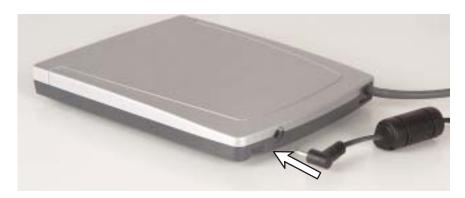
**2** Connect the IEEE 1394 cable from the drive to the jack on the tablet PC or FlexDock.
