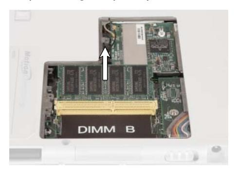
11 Hold the new or replacement module at a 30-degree angle and press it into the empty memory slot. This module is keyed so it can only be inserted in one direction. If the module does not fit, make sure that the notch in the module lines up with the tab in the memory bay.
